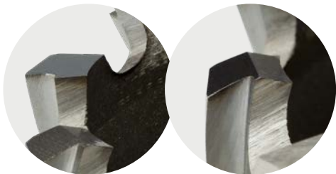
HSS cutters have two different teeth
